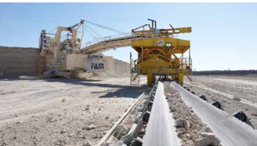
Excavator in the chalk pit with conveyor belt to the cement factory
