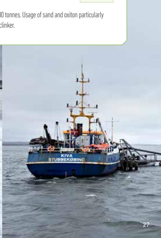
Sand from navigation channels pumped from dredgers to drainage basins ashore
