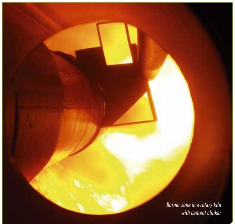
*Burner zone in a rotary kiln with cement clinker*
